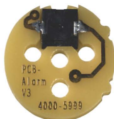
PCB-Alarm Installing Piezo function for H5XXX.1A4 H5XXX.1P
