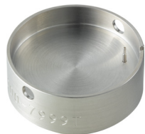
Movement holder Removing setting stem H7XXX.1T
