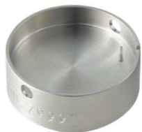
Movement holder Removing setting stem H7XXX.1T
